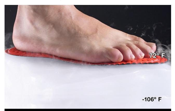
Even at a pressure of 15 psi, Aspen Aerogels' insulation retains over 85% of original thickness and over 97% of its original thermal performance.
