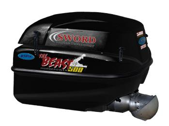
propulsion systems, introduces a state-of-the-art 500 hp JetPac. This revolutionary outboard features a heavy-duty, 7-liter GM LS7 engine, making it the most powerful outboard engine in the world.
